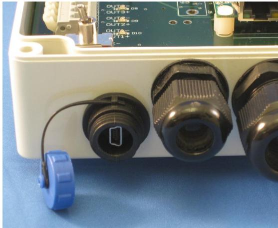
**The function of the USB connector is controlled by S2 and S4 settings.**
