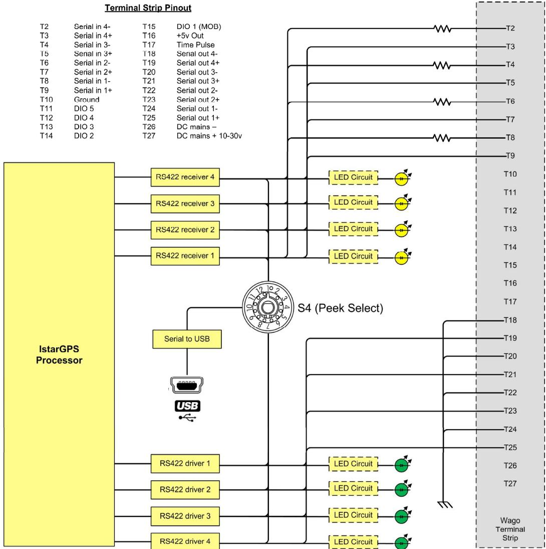
Figure 17 Serial to USB data output signal flow (shown in unbalanced output, terminated input configuration)
