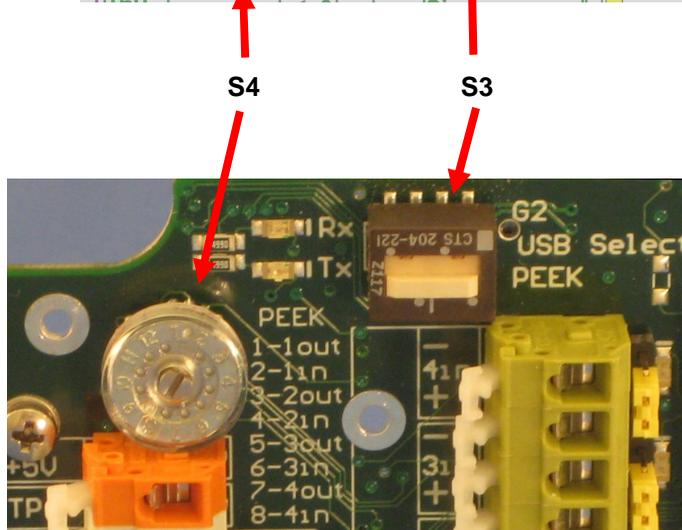
Figure 16 USB port selector S3 and Peek selector S4
