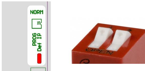
Figure 37 Flash Programming Switch S1 and location
