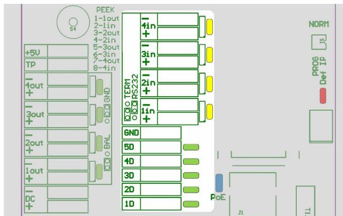
Figure 19 Digital I/Os and Serial Inputs
