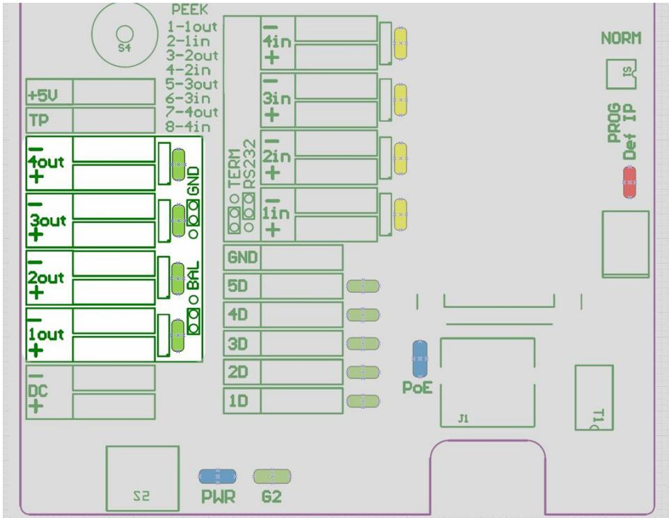
Figure 7 NMEA outputs and status LEDs
