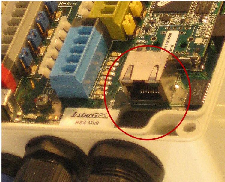
Figure 11 RJ45 Ethernet connection
