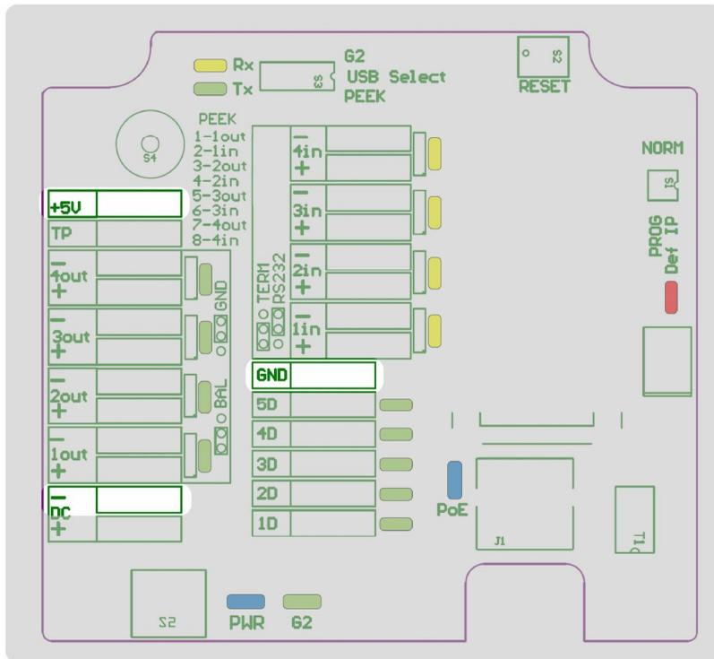
Figure 19a 5 Volt output and ground reference locations
