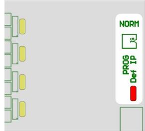
Figure 13 IP Reset and Default IP LED
